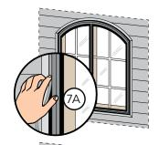
B. Apply a bead of high quality exterior grade sealant to the entire perimeter of the window.
